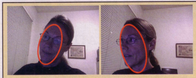
FIGURE 1. OpenCV's face tracker in action. It's able to follow a face as it tilts to one side and during a turn to profile.
