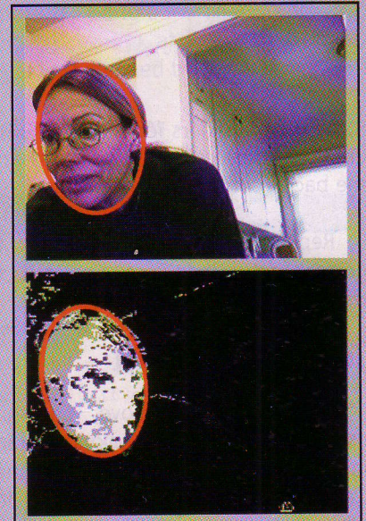
FIGURE C. The normal and face-probability views as Camshift tracks my face. In the face-probability view, black pixels have the lowest value, and white, the highest. Gray pixels lie somewhere in the middle.
